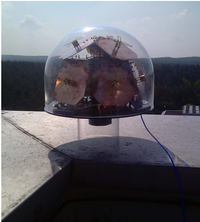
Hemispherical Scan Antenna by Prof. Jan Hesselbarth, UNI Stuttgart L-Band
